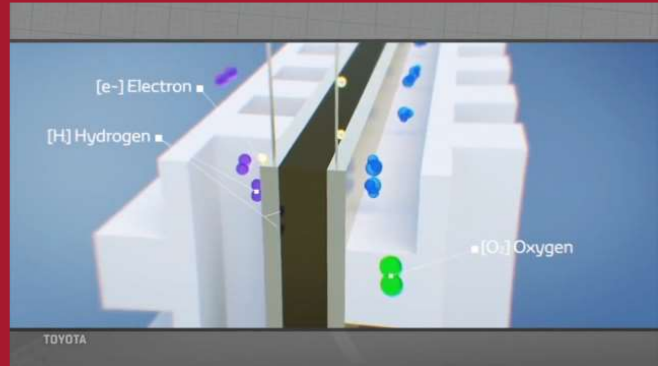
Basic diagram of a PEMFC.
