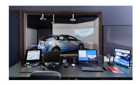
"Drivers' response to warnings/ information provided by in-vehicle applications/ systems" (TAR16/18) <u>Virtual environment</u> - complete control of road layout, traffic, and road design and collection of various performance measures (speed, SDLP, brake reaction time etc.)
