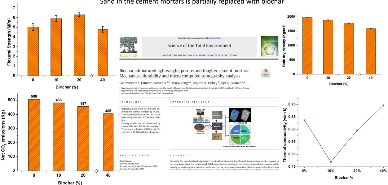
Sand in the cement mortars is partially replaced with biochar
